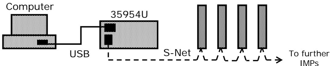
Connection between the computer and the **35954U** is by USB cable. From that point, the wiring to the IMP network conforms exactly to the S-Net requirements for cable type and length. As with the S-Net, the **35954U** may be positioned at the end of the cable, or centrally to meet physical needs.
