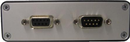
The rear panel supports two 9 pin DIN connectors for power and communications.
