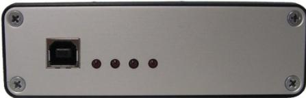
The front panel supports the USB type B connector (USBv2.0) and the 4 status LEDs.
