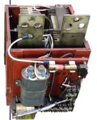
Upon arrival, bus bars are corroded and dirty, wiring is degraded, fuses and capacitors are of questionable integrity, and general condition is poor, reflecting a hard working life.
