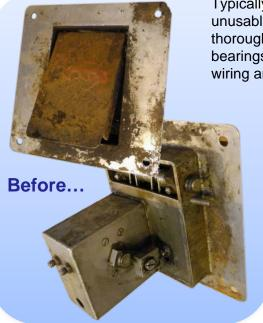
Typically, units arrive in poor condition - totally seized and unusable; they are then completely disassembled, thoroughly cleaned and de-scaled, and are fitted with new bearings, bearing blocks, hardware and seals, prior to rewiring and calibration.
