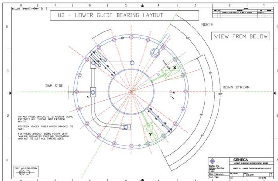
Fig 8: Constructed scale drawing of Lower Guide Bearing Cover Plate
