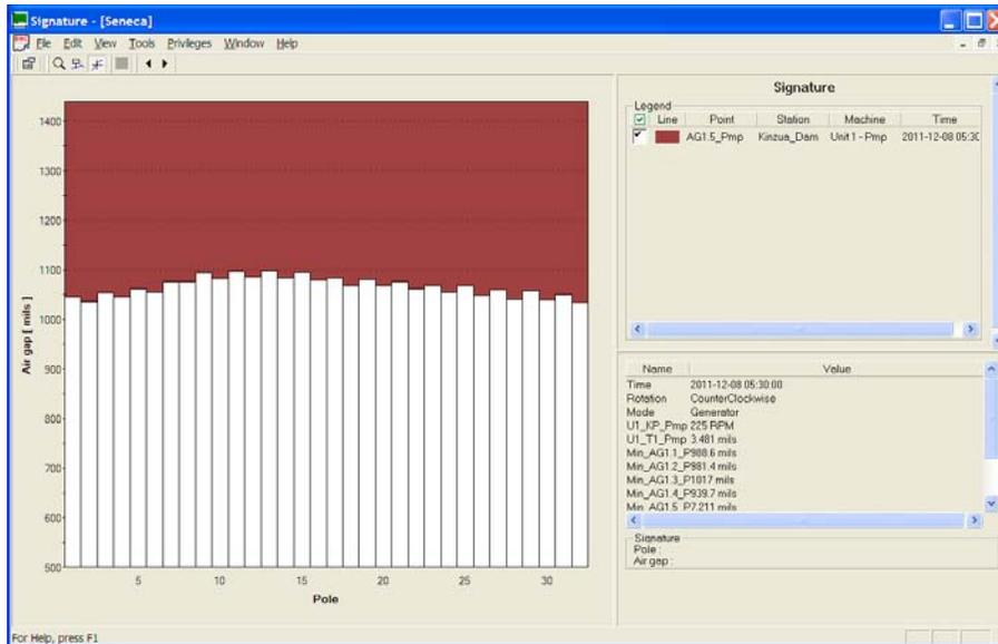
Fig 16: Signature / AG1.5 in Pumping Mode / CCW
