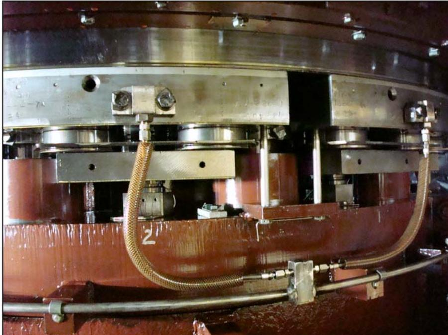
*Fig 6: Unit 1 (2) thrust bearing detail*
