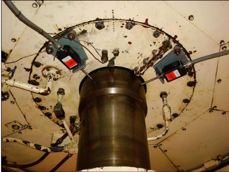
*Fig 10: New X/Y Probes fitted to LGB Cover*
