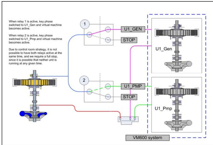
Fig 14: Key Phase switching for units 1 (U2 identical)
