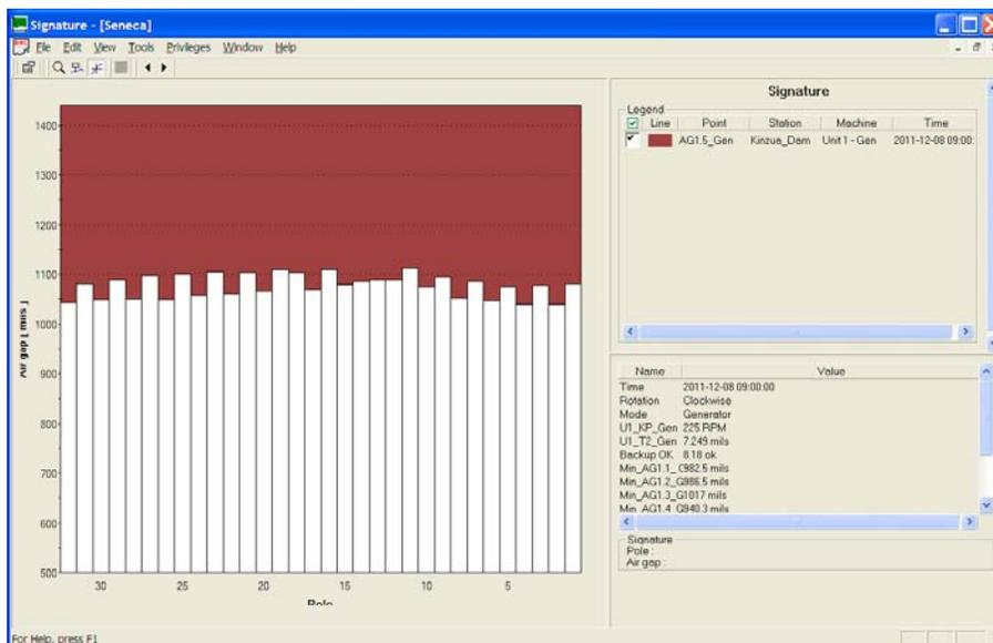
Fig 17: Signature / AG1.5 in Generating Mode / CW
