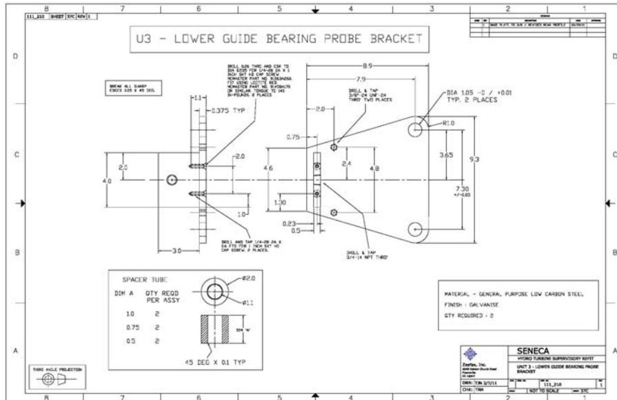
Fig 9: Lower Guide Bearing Detail
