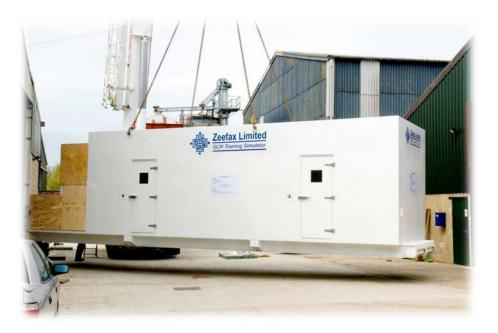
The 40 foot long, self contained simulator includes operator and instructor workstations, where trainee activities can be viewed and assessed, and known faults can be selectively introduced during tests and assessments. The Power Control Room also contains a PLC training station, complete with graphical display, facilitating training in the use of PLC controlled systems, including troubleshooting and component replacement.
